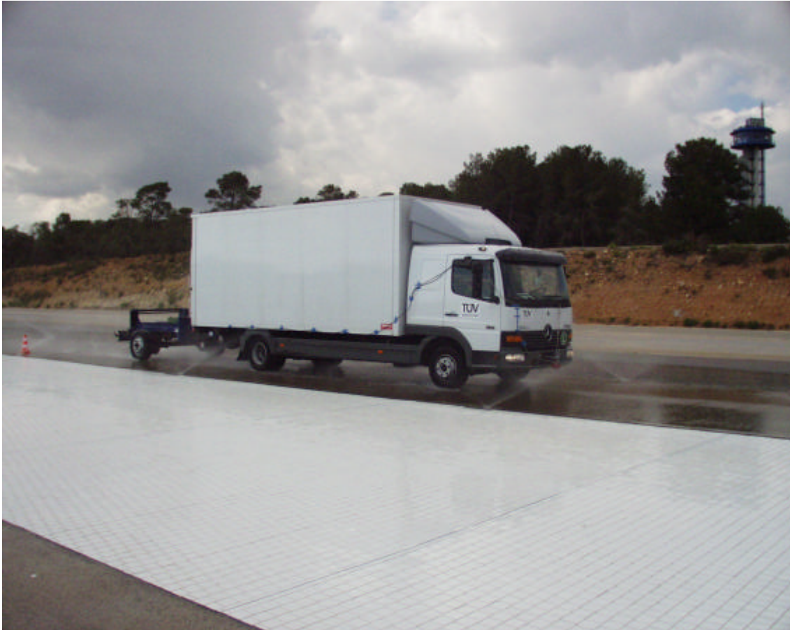
Figure 3: Braking on a wet surface with test trailer, tire size 215/75 R17.5
