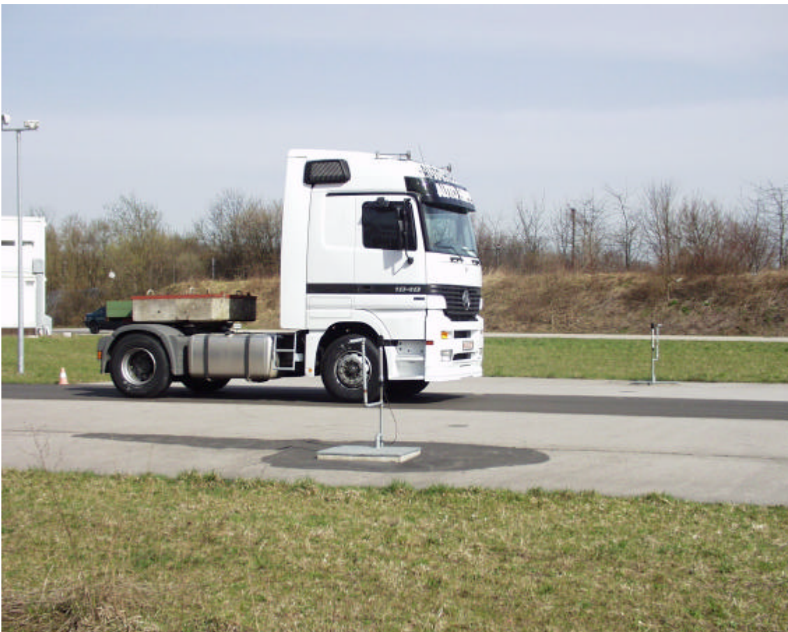
Figure 2: Noise measurement conducted for MB Actros, tire size 315/80 R22.5
